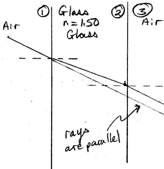
As we saw in problem 3, the amount of refraction going into air medium (glass) is compensated by refraction @ the 2<sup>nd</sup> surface.
