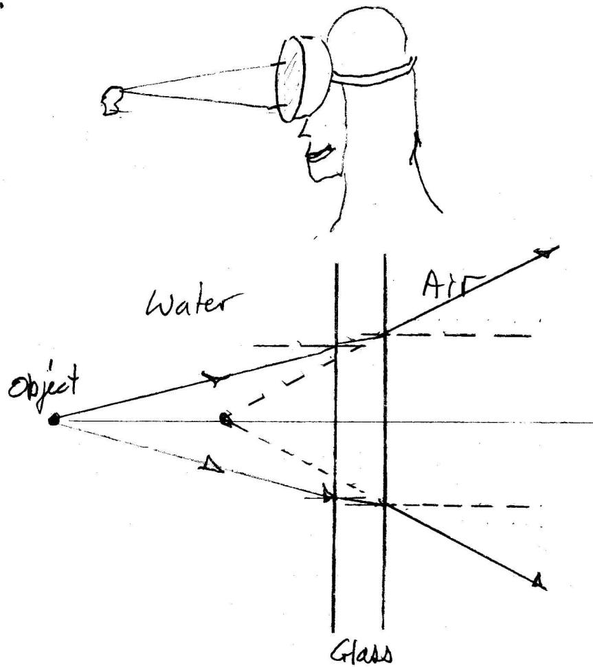
Because the light rays will bend away from the normal compared to initial ray the object will appear closer than is really is.
